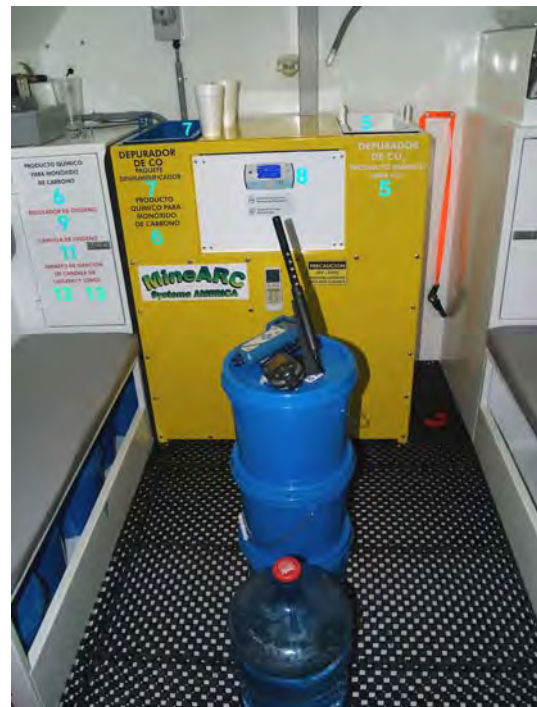
Monitoring equipment placement within refuge chamber
