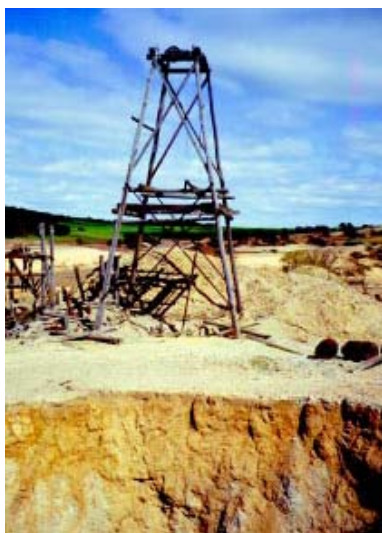
Un-capped shaft with sinkhole in foreground.
