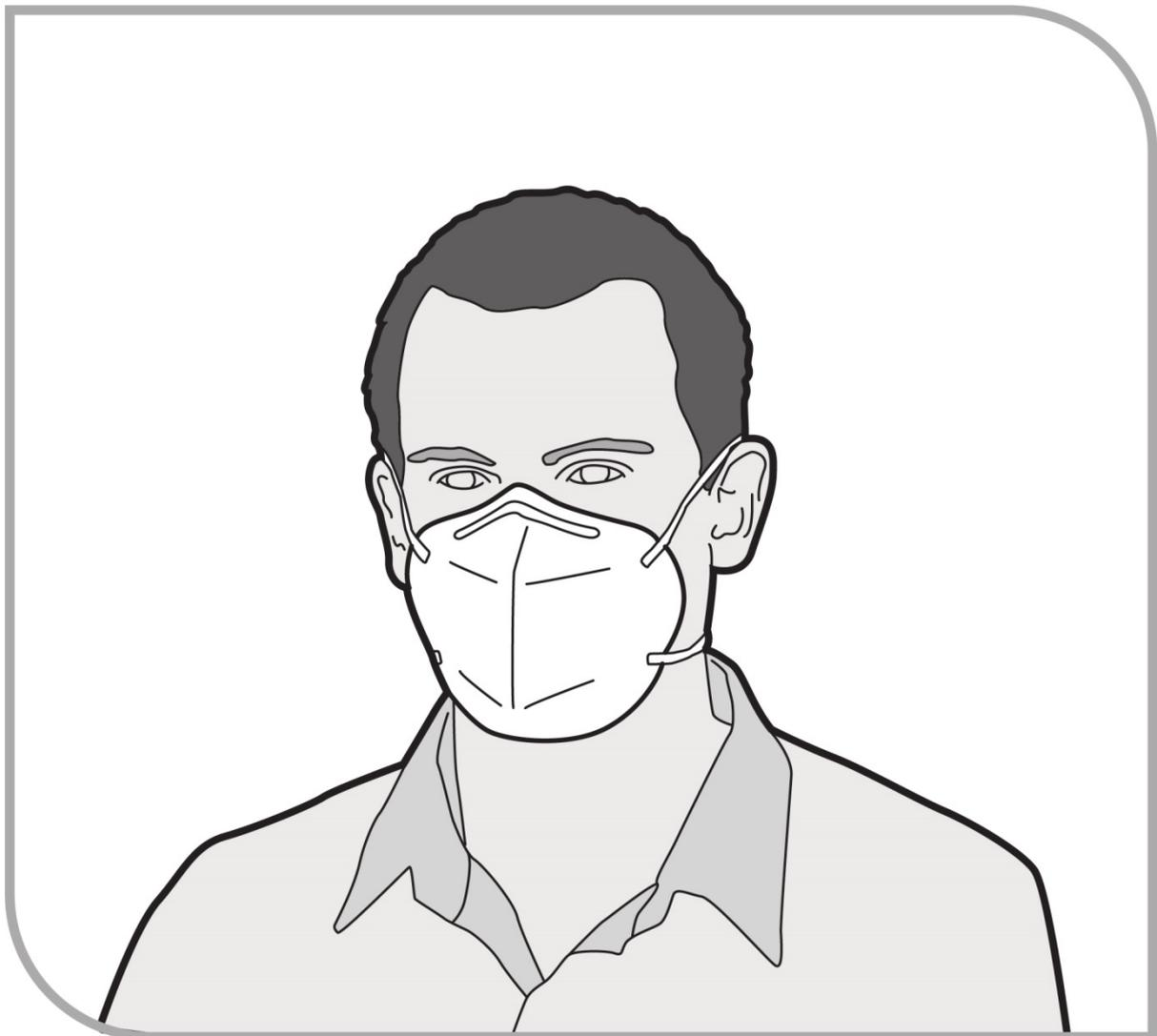
**Figure 9** Disposable, half-face particulate respirator
