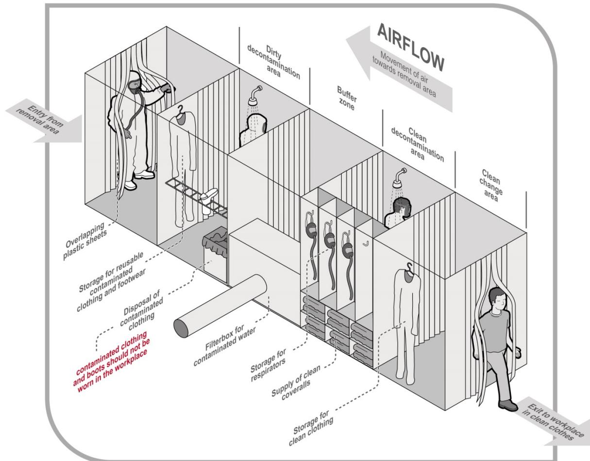
Figure 4 Decontamination unit
