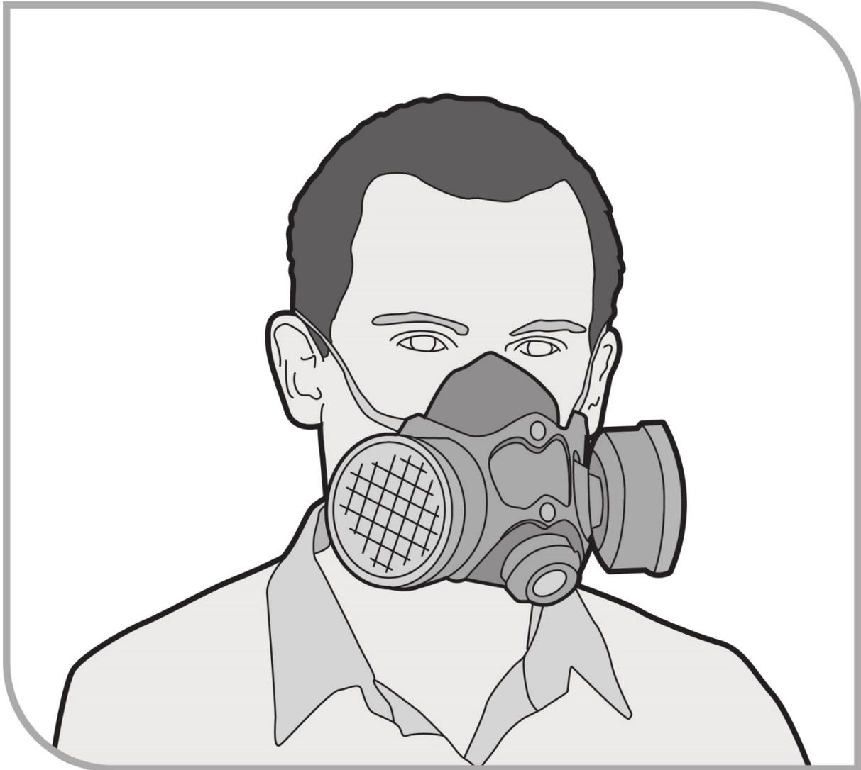
**Figure 10** Half-face particulate filter (cartridge) respirator
