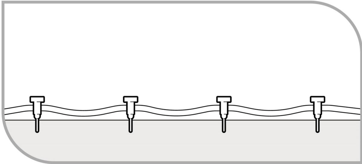
**Figure 3** Saturating asbestos using the water injection method
