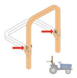
A ROPS has a limited lifespan and should be inspected regularly to identify signs of physical deterioration, for example dents, rust or cracks. The structural integrity of a ROPS can be impaired by continuous impact corrosion and this may be indicated by deformation or cracking of the structure. A ROPS in poor condition should be replaced.
