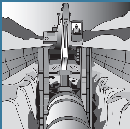
FIGURE 6 Extending trench shields above the excavation
