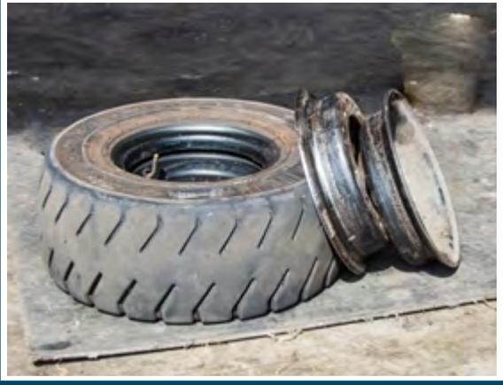
**Figure 16** Use of standard nuts (attaching wheel to hub) and 'D' section bolts (securing two parts of a divided wheel together)
