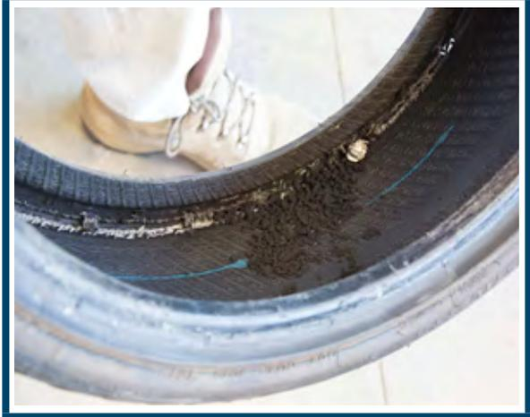
**Figure 7** Delaminated outside tyre
