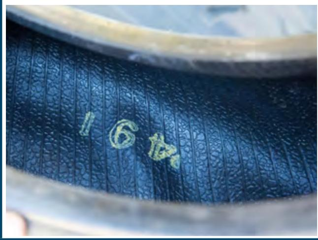
**Figure 6** Damaged side wall which can cause zipper failure
