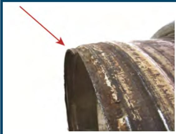
Figure 2 shows a wheel similar to Figure 1 with cracks and excessive corrosion which could not be observed while it is still fitted on the vehicle.
