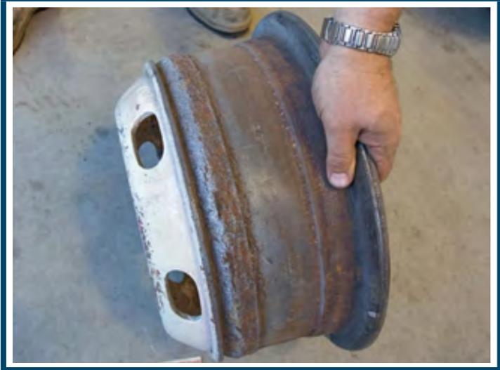
**Figure 10** Shows surface rust (not pitted) can be removed with a powered wire brush
