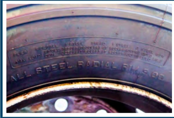
Figure 4 shows the four digit code for the week and year the tyre was manufactured. The tyre in the figure indicates that the tyre was manufactured in the 13th week of 2012.
