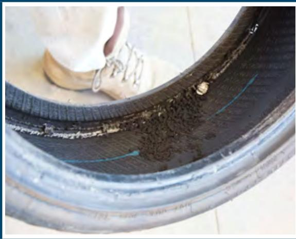
**Figure 7** Delaminated outside tyre
