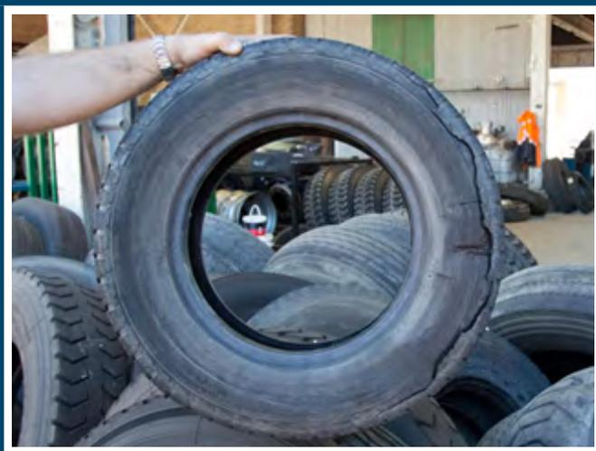
**Figure 8** The wall of the tyre is slightly distorted
