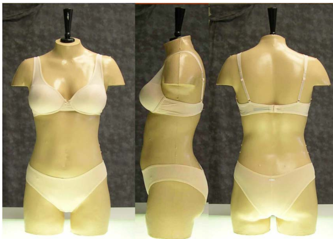
Figure 15 An apparel manikin made from a 3-D body scan.
