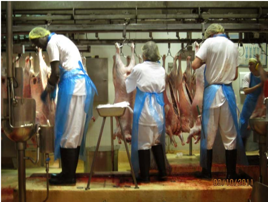
Figure 23: A shared fixed height workstation in an abattoir that attempts to accommodate three workers of different heights.
