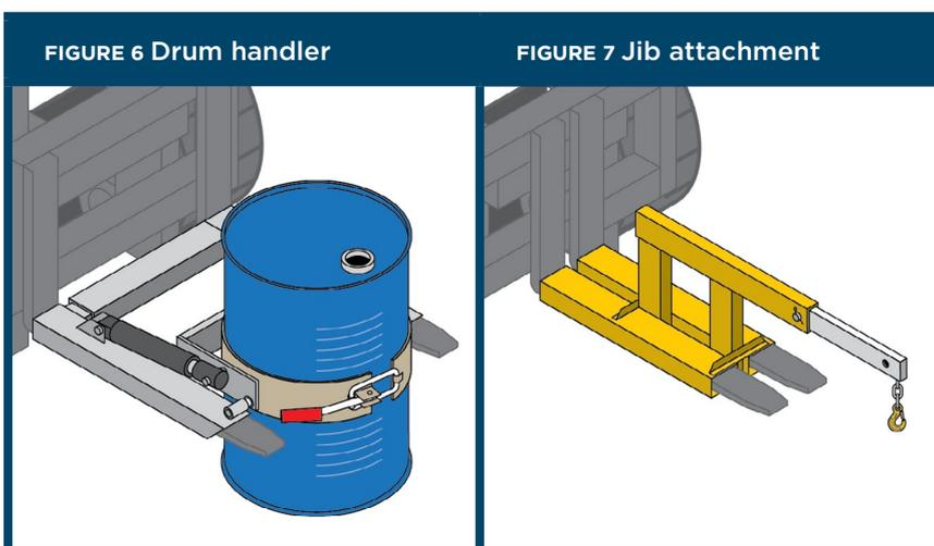
When choosing an attachment, check with the manufacturer or supplier of the industrial lift truck whether it can be used safely. If you fabricate an attachment, it must be designed by a competent person, for example an engineer, for the industrial lift truck it is to be used with. Specific training and supervision in the use of an attachment should be provided as necessary.
