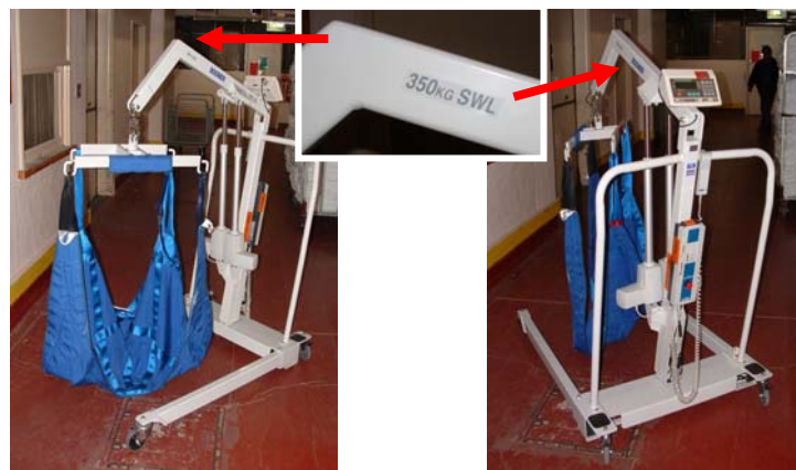
Front and rear views of a bariatric lifting machine which includes in-built scales. Inset: Indication of the safe working load label
