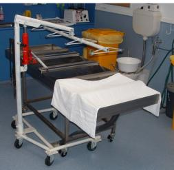
The lifting device was designed and built in-house. The device has a lifting arm from which straps are suspended and passed around the deceased. The device employs bottle-jack to raise the arm. No safe limits have been determined. While the bottle jack has a stated load limit, the load imposed by the lift at the end of the lifting arm will be greater than that at the point of application of the jack force. The load imposed by the lifting of any body is therefore unknown.
