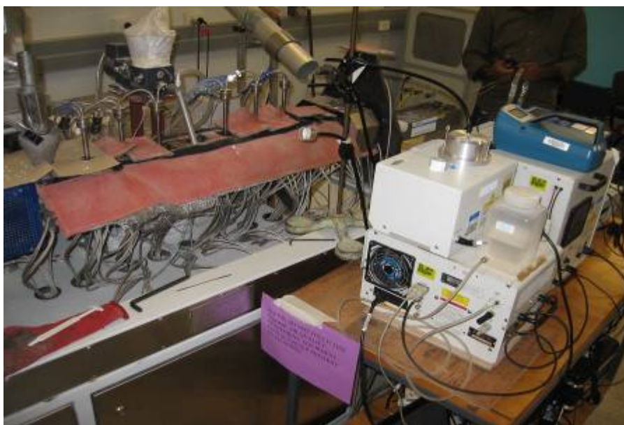
Figure 6: Configuration of measurement equipment, with sampling manifold, relative to the location of the extruder machine.
