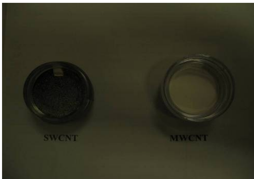
Figure 34: photograph of the open face cassettes containing the filters used to capture nanotubes. The SWCNT filter on the left shows significantly more particle deposition than the MWCNT filter on the right.
