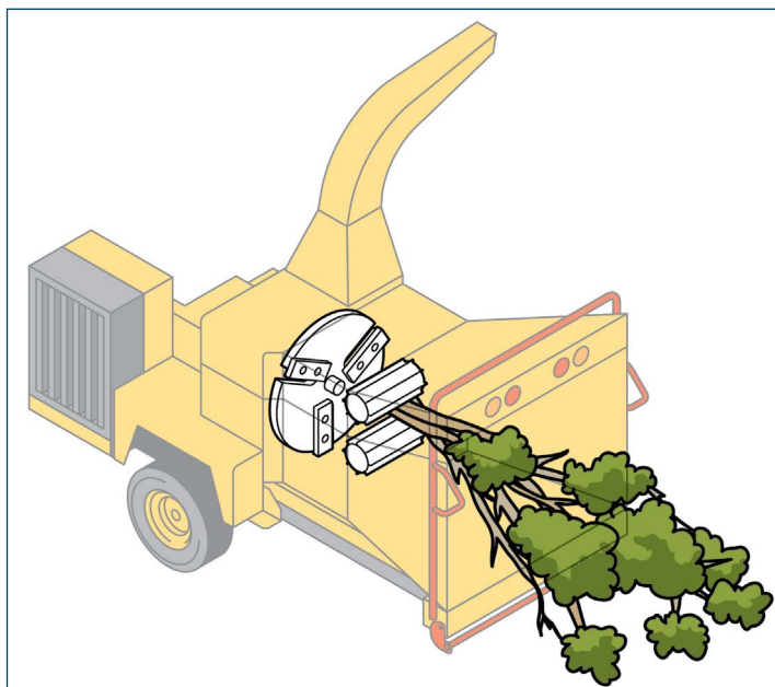
Figure 6 Disc-type wood chipper showing in-feed rollers and cutting disc
