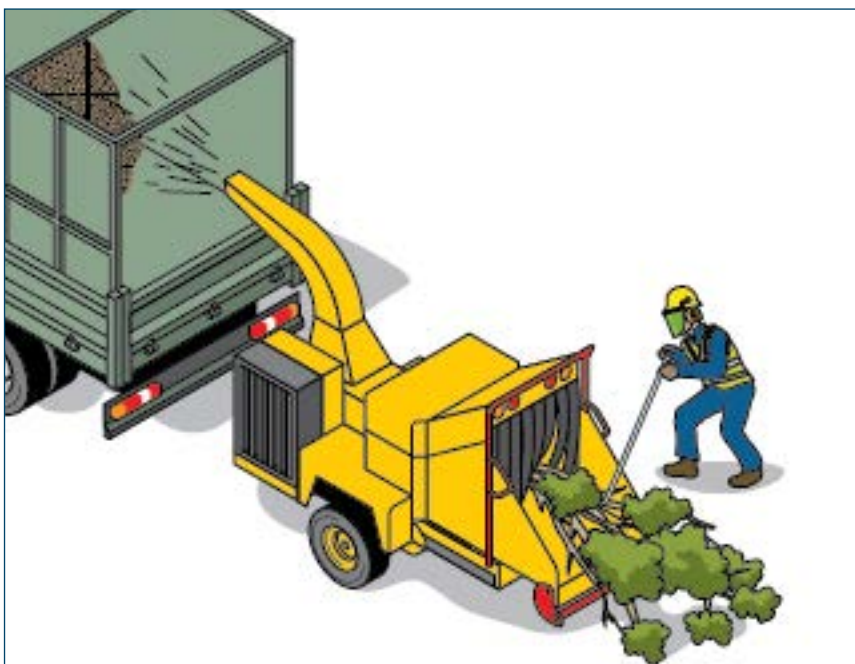
Figure 5 Using a push-stick to feed shorter branches into a wood chipper
