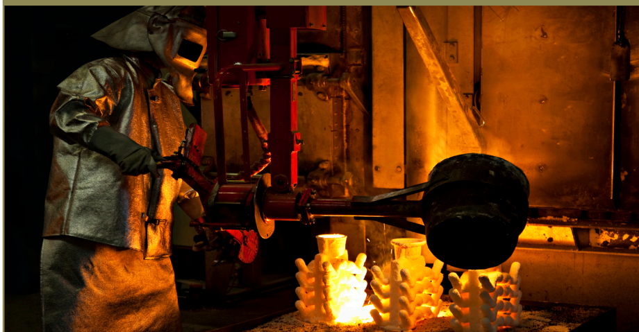
Figure 7 Worker wearing primary PPE pouring liquid metal into moulds
