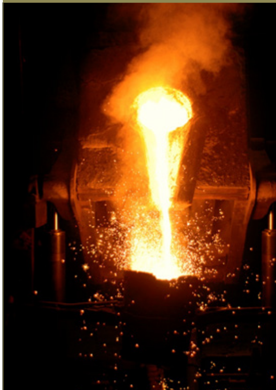
FIGURE 1 POURING LIQUID METAL FROM A FURNACE - SHOWING MOLTEN METAL AND HEAT HAZARDS
