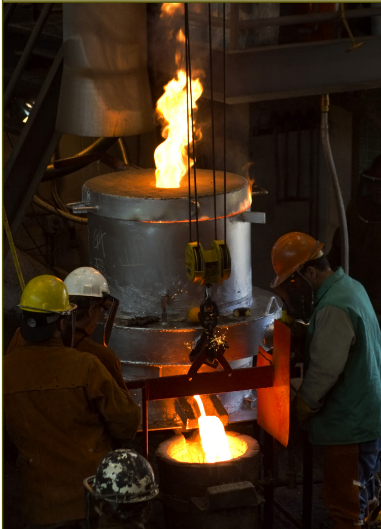
Figure 9 Workers pouring liquid metal wearing PPE
