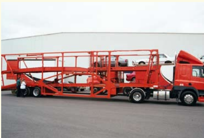
Car-carrier where the frame extends to a sufficient height to provide a barrier against falls. The frame of many car-carriers extends only to the height of the floor of the top deck leaving the driver walking alongside vehicles with no fall protection.
