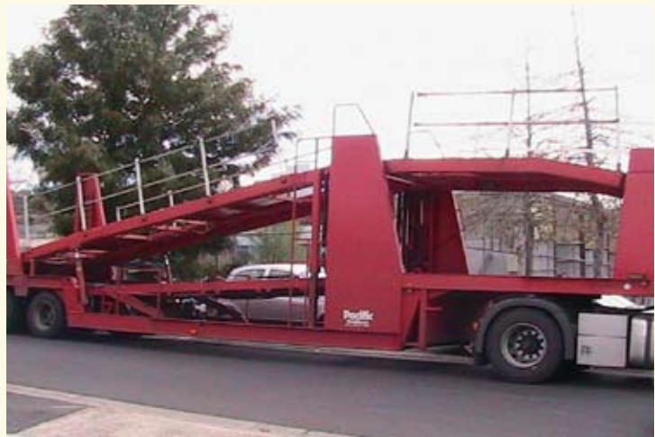
Car-carrier with fall protection railings
