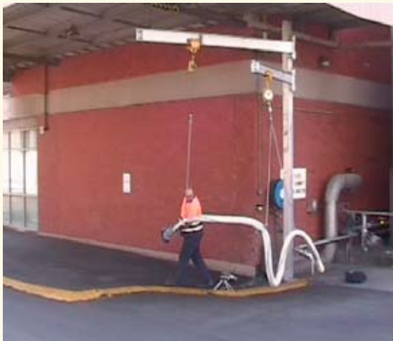
Load balancing for a heavy liquid receiving hose
