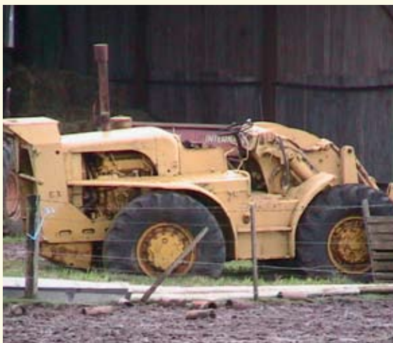
Loader without roll over protection. Photo: J.Culvenor
