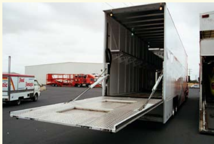
Enclosed car-carrier with fall protection provided by side walls
