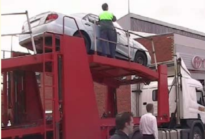
Accessing the vehicle on a car-carrier with the railing fitted.
