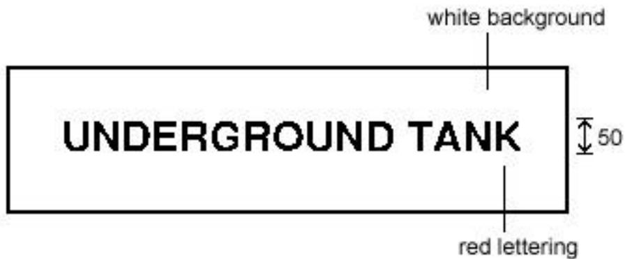
This placard is complemented by a composite warning placard (Top section of a Transport Emergency Information Panel (EIP)).
