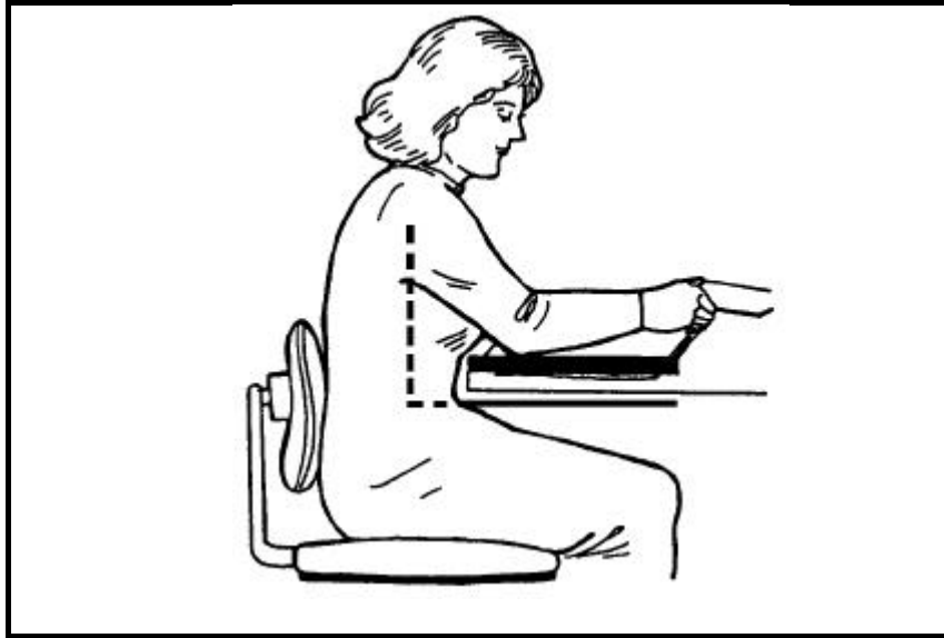
Figure 7 The work level should be above the elbow if work requiring precision is done on a level desk, for example, assembly work, as demonstrated in this figure. The work level chosen should be a compromise between the visual demands of the task and a suitable position of the arms.
