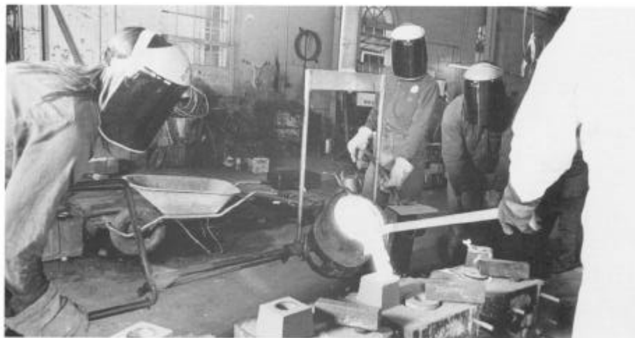
When pouring molten metal, appropriate personal protective equipment and protective clothing should be worn
