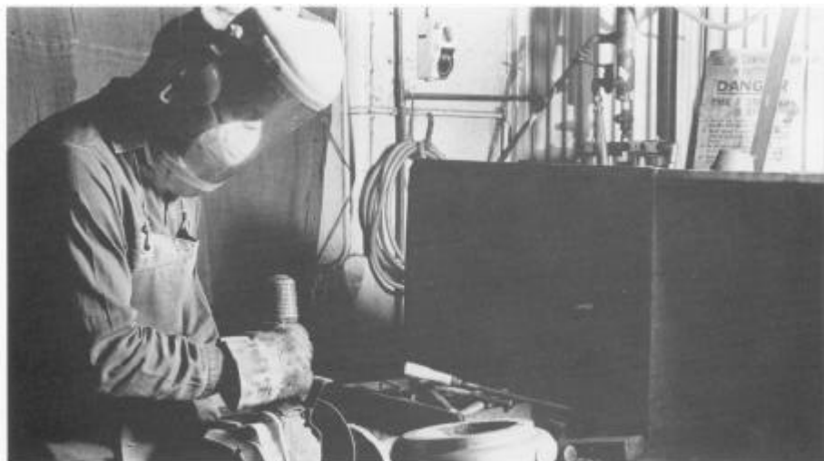
During dressing and cleaning of the castings, eye protection, face shields, goggles, earmuffs, respirators and gloves should be worn
