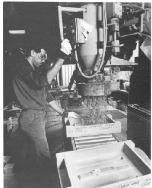
When working with sand and binder in mould or core making, use eye protection and gloves
