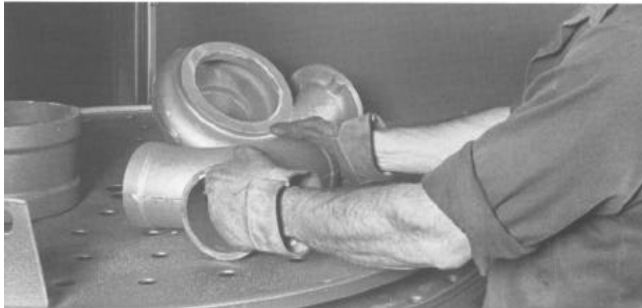
Gloves should be worn when handling castings to reduce the likelihood of injuries to the hands
