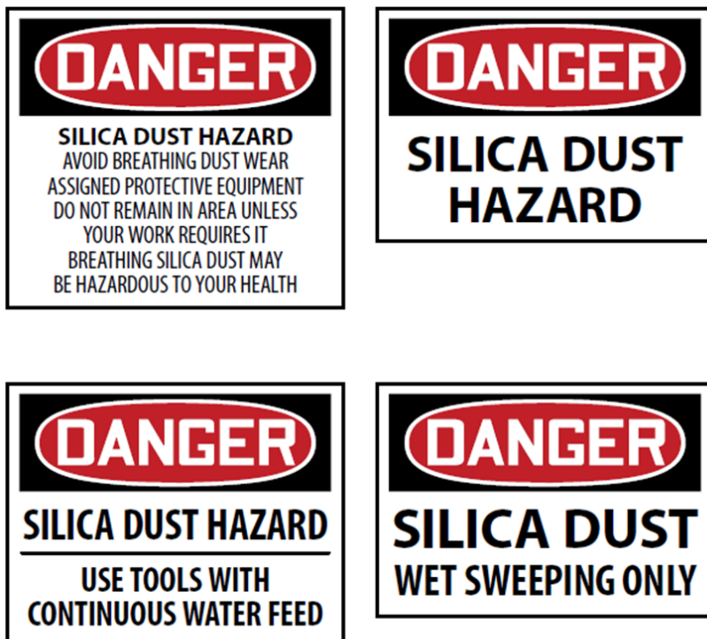
Figure 6 Examples of dust hazard signs
