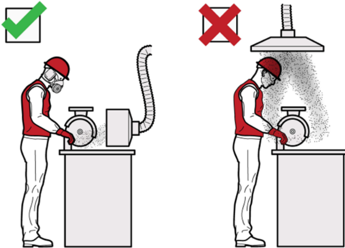
Figure 5 Examples of using local exhaust ventilation
