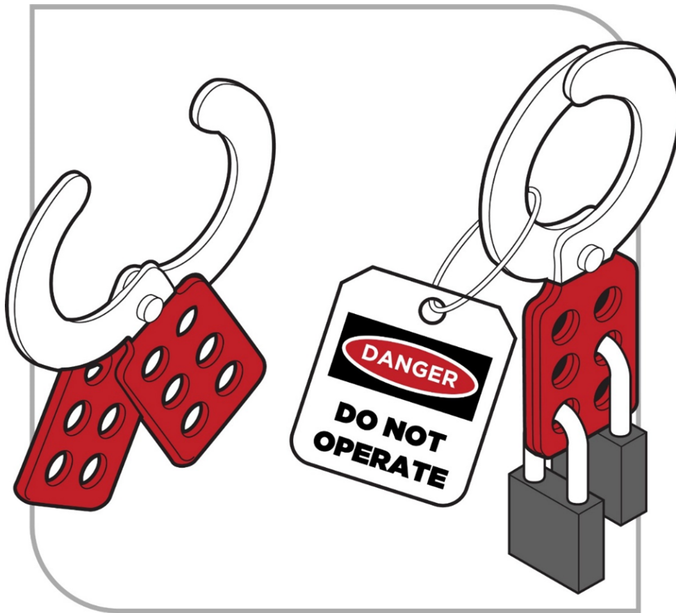
Figure 3 Example of tag and lockout with padlocks
