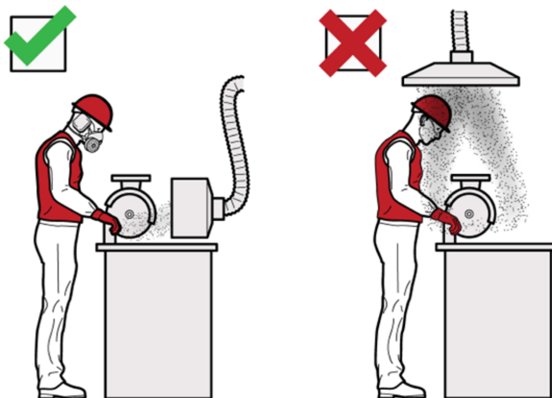
Figure 5 Examples of using local exhaust ventilation
