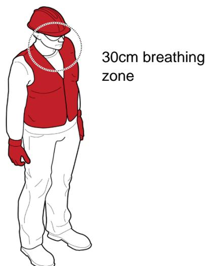
**Figure 1:** Worker breathing zone from which personal samples must be taken
