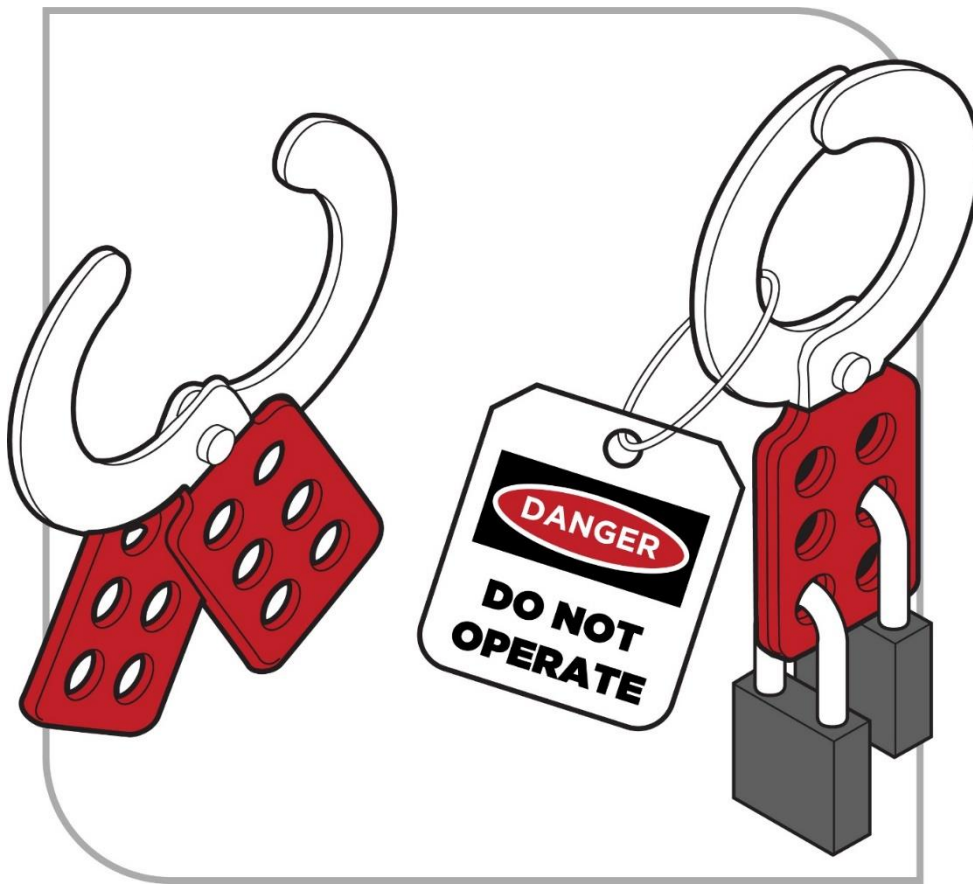
Figure 3 Example of tag and lockout with padlocks
