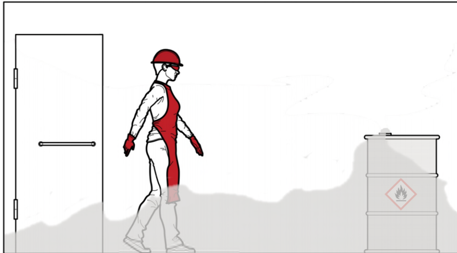
Figure 2: Stored flammable liquids may create hazardous vapours
