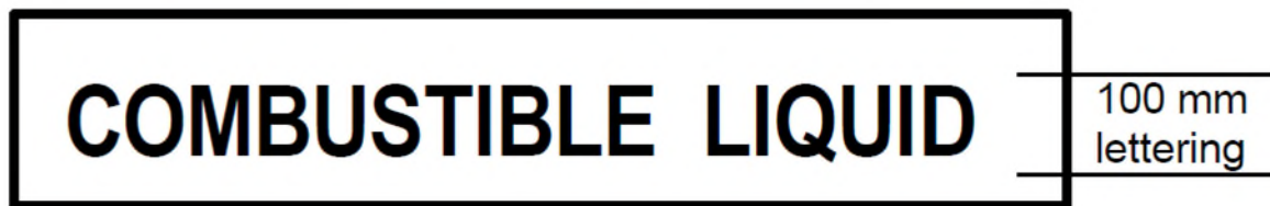
Figure 5: Package storage placards for Category 4 flammable liquids
