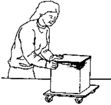
**Figure 44 - Rolling platform to avoid lifting**
