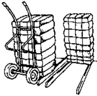
Figure 35 - Rails enable trolleys to slide under loads
