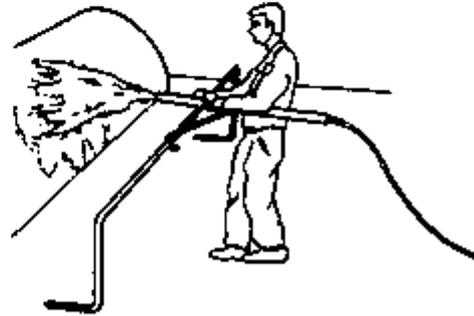
Figure 30 - Use structures to absorb reaction forces
