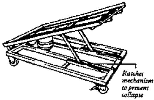
**Figure 45 - Rolling platform with tilt mechanism**
