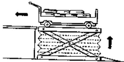
Figure 39 - Adjustable height platform reduces lifting
