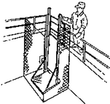
**Figure 61 - Elevator for transporting goods between floors**
