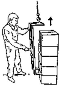
**Figure 59 - Lifting device for moving boxes and crates**
