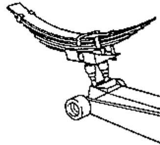
**Figure 34 - Support weight by use of jack**
