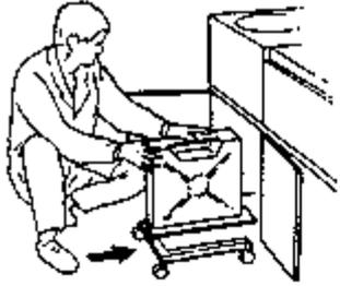
Figure 27 - Simple trolley avoids awkward handling
