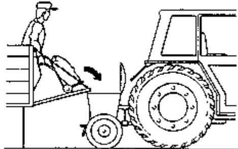
**Figure 19 - Gravity feed principle to avoid lowering**
