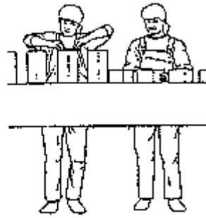
Figure 24 - Tilt objects to reduce work height
