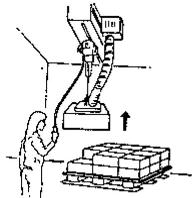
Figure 58 - Vacuum lifter for material handling
