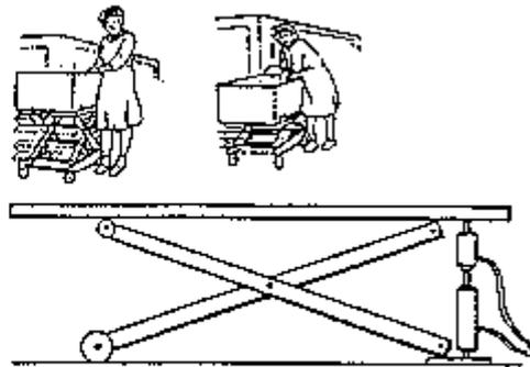
Figure 50 - Adjustable scissor table for different work heights
