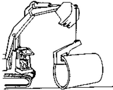
**Figure 52 - Using c-hook to move cylinders and pipes**
