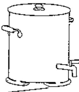
**Figure 20 - Tap avoids lifting to empty**
