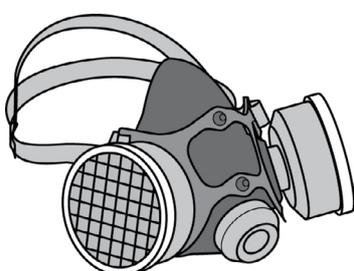
Respirators need to be properly stored, inspected, cleaned and maintained. Workers should be trained and fit-tested to use a respirator.
