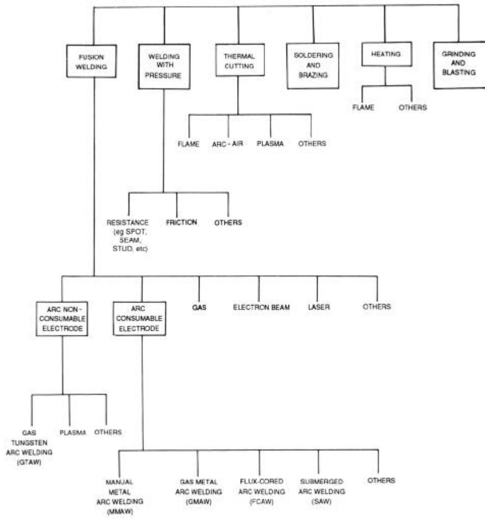
Figure 1. Welding and allied processes
