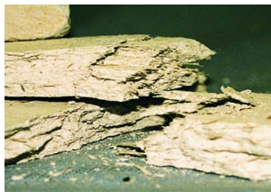
Broken crumbled friable asbestos
